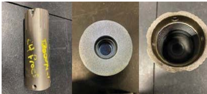
Successful after 24 stages frac, 600 tons of sand at 6.5 m 3 /min comparing to other surface treatment technologies.
